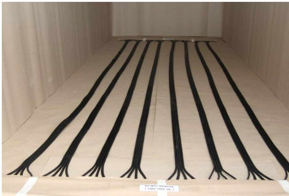
Steam heating tubing laid out across the container floor prior to flexitank installation.
